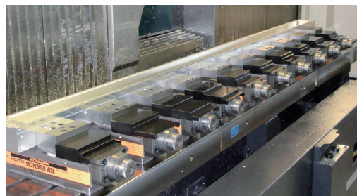
▲3mリアテーブルのM/Cにバイス10台を並列仕様で搭載 ▲On the 3 m linear table, 10 vises are mounted with the parallel specification.
