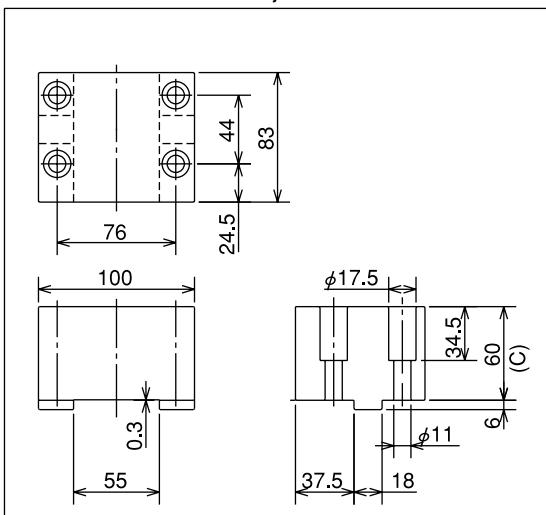
2) Forming soft jaws are stocked at our company as shown in the Soft Jaw Dimension Table. The material is S45C. It is possible to partially harden these soft jaws.
