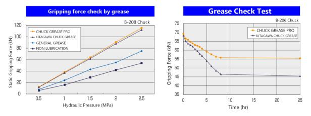
The graphs show the grease performance, not the condition of using Chuck. Please refer to Chuck specification table for the condition of Chuck.
