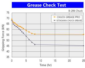
\*The graphs show the grease performance, not the condition of using Chuck. Please refer to Chuck specification table for the condition of Chuck.
